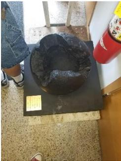
**Object Name:** 15-inch shell; fuse; welded back together from nine pieces
